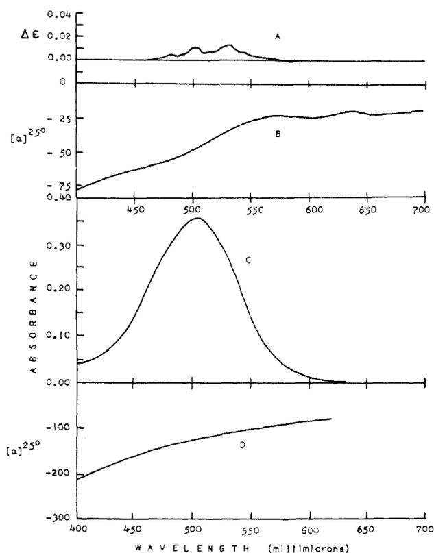
Figure 1.—A: circular dichroic absorption. B: optical rotatory dispersion of  $[\text{Co}(\text{NH}_3)_5(l\text{-menac})](\text{NO}_3)_2$  (I) in water at  $25^\circ$  ( $c = 0.12$  g/100 ml, 10-cm cell). C: absorption spectrum of I in water at  $25^\circ$  ( $c = 0.24$  g/100 ml, 1-cm cell). D: optical rotatory dispersion of sodium *l*-menthoxyacetate in 50% ethanol-water at  $25^\circ$  ( $c = 0.12$  g/100 ml, 10-cm cell).
